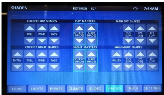
Figure 12-11: Day/Night Window Shade Control
