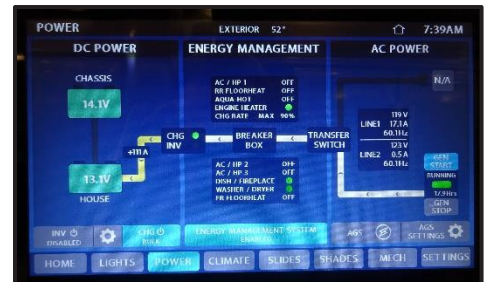
Figure 9-12: Energy Management System
