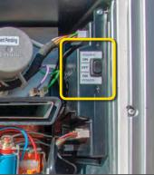
Figure 73. Truma Water Heater Control Dial and On/Off Switch
