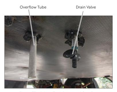
Figure 75. Water Tank Drain and Overflow
