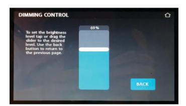
Figure 34. Spyder Dimming Control Screen
