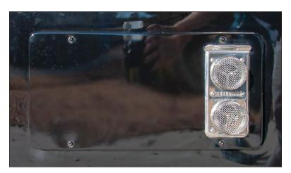
Figure 109. Furnace Vent (Shown with Customer Supplier Insect Screens)
