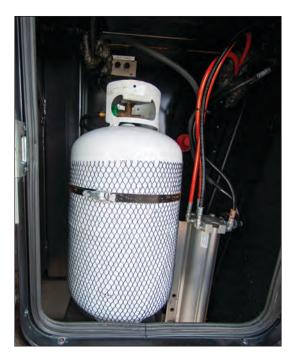
Figure 78. Propane Gas Cylinder
