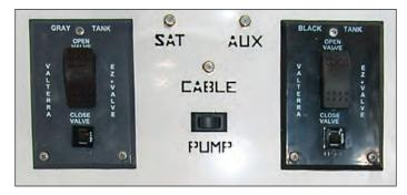
Figure 64. Black and Gray Tank Drain Valve Switches
