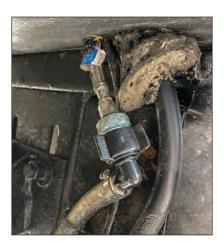
Figure 72. Ice Maker Drain behind Galley Slide
