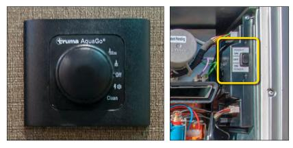
Figure 56. Truma Water Heater Control Dial and On/Off Switch
