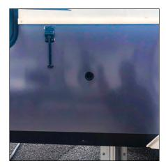
Figure 19. Spare Tire Winch Access Hole
