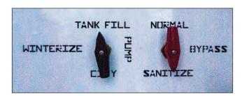
Figure 59. Sanitizing the Fresh Water System
