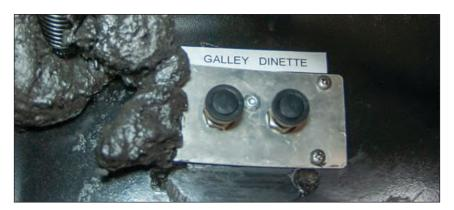
Figure 117. Hydraulic Slide Bleed Valves
