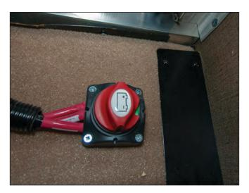
Figure 31. Battery Disconnect Switch
