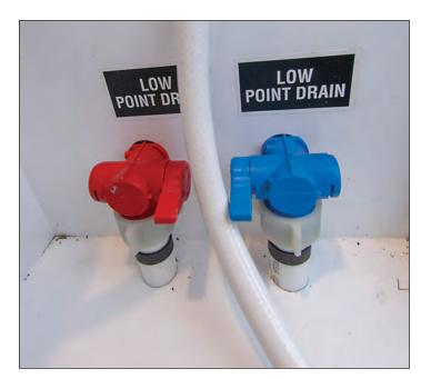
Figure 68. Low-Point Drains located under the RV
