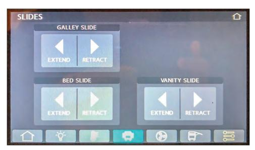
Figure 115. Slideout Controls
