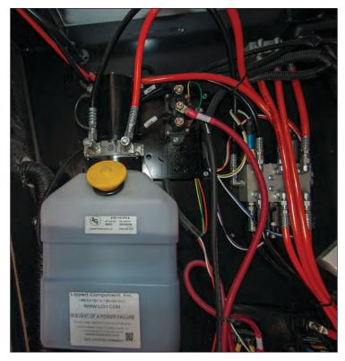
Figure 116. Hydraulic Reservoir for Slides and Leveling
