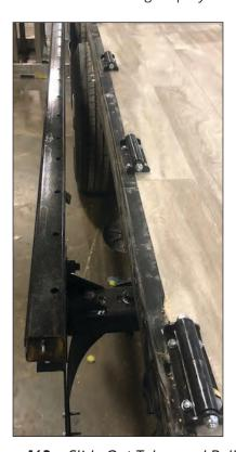
Figure 143. Slide Out Tubes and Rollers
