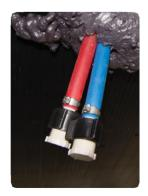
Low-Point Drains located under the RV
