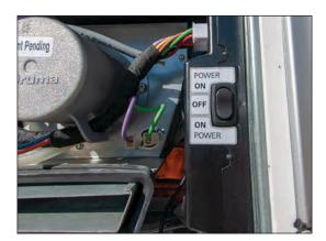
Figure 46. Truma Water Heater Exterior On/Off Switch
