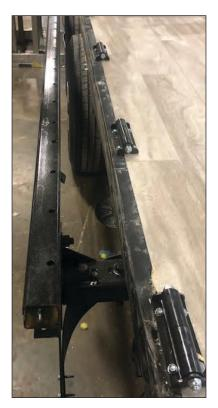
Figure 144. Slide Out Tubes and Rollers
