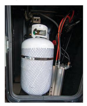
Figure 79. Propane Gas Cylinder
