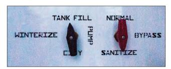
Figure 60. Sanitizing the Fresh Water System
