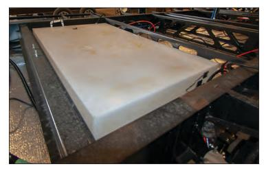
**Figure 40.** Fresh Water Holding Tank
