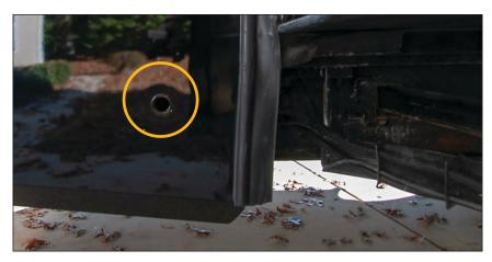
Figure 20. Spare Tire Winch Access Hole
