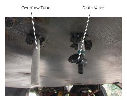
Figure 76. Water Tank Drain and Overflow
