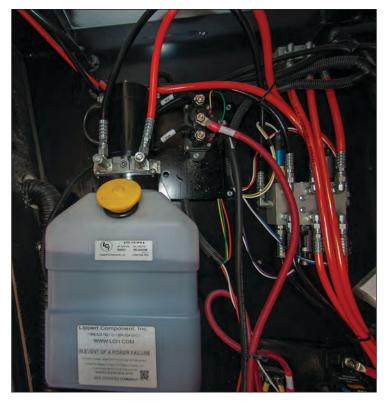
Figure 117. Hydraulic Reservoir for Slides and Leveling
