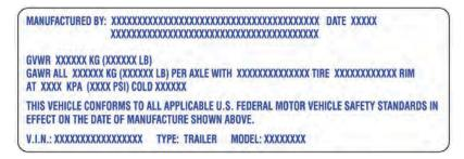
**Figure 8.** Federal Certification Label (Example) (Located on the Forward, Off-Door-Side Exterior)
