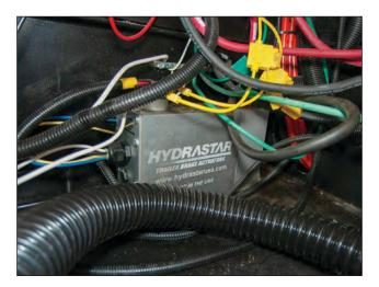
Figure 12. Brake Actuator (for optional Disc Brake System)
