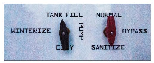
Figure 37. Sanitize the Water Tank before First Use
