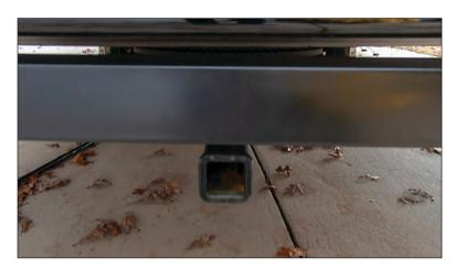
Figure 130. Bolt-On Hitch
