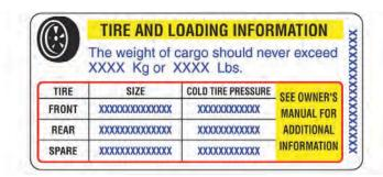
Figure 10. Tire and Loading Information Label (Example)
