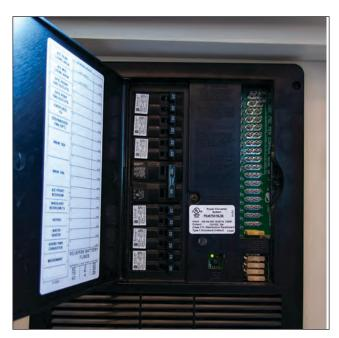
Figure 31. 12V Fuse Panel
