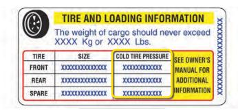
Figure 16. Tire and Loading Information Label (Example)
