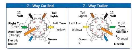
Figure 13. 7-Way Wire Harness/Connector Plug
