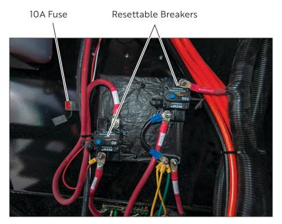
Figure 142. 10A Fuse and Resettable Breakers for Jacks/Leveling System
