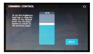
Figure 35. Spyder Dimming Control Screen
