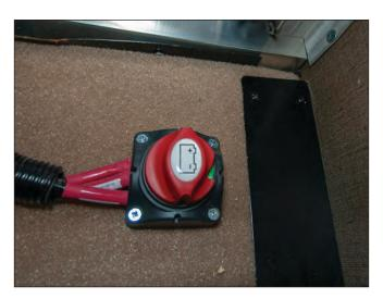
Figure 32. Battery Disconnect Switch
