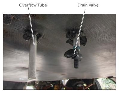
Figure 41. Water Tank Drain and Overflow
