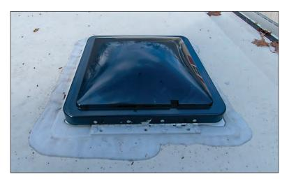
Figure 141. Roof Sealant
