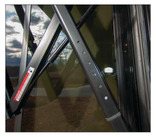
Figure 128. Awning 6-point Adjustment Pins
