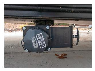
Figure 66. Sewer Outlet Connection (Termination Valve)
