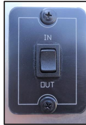
Figure 10-4: Electric Slide Tray Switch on Cargo Door
