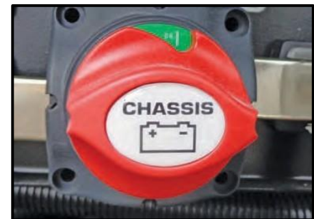
Figure 8-6: Engine Battery Disconnect Panel Switch
