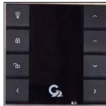
Figure 13-2: Awning control switch
