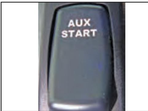
Figure 8-2: Auxiliary start switch
