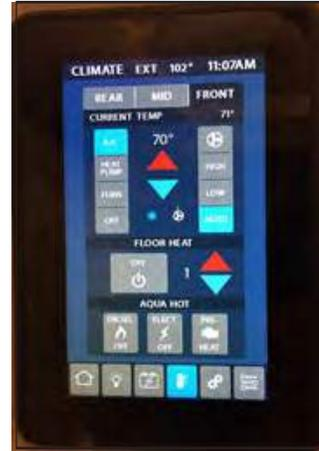
Figure 3-9: A/C Thermostat control page on 5" panel
