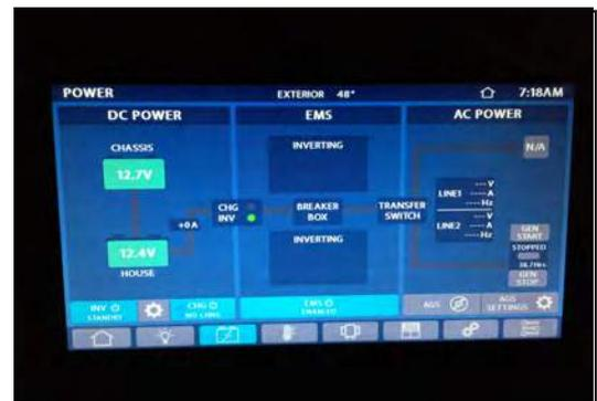
Figure 8-11: Converter/Inverter control screen
