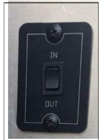
Figure 9-3: Electric Slide Tray Switch on Cargo Door
