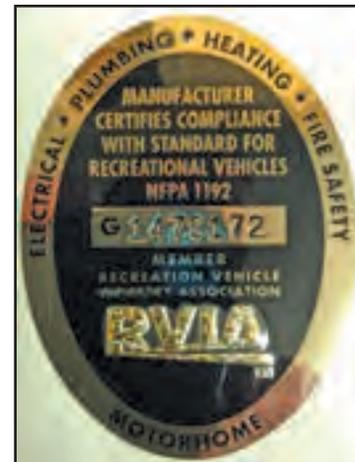
Figure 1-2: RVIA Label located on the outside of the motorhome
