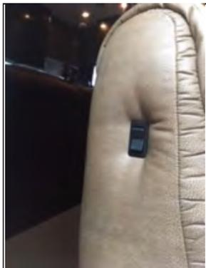
Figure 9-2: Slide-out switch on passenger and driver seat
