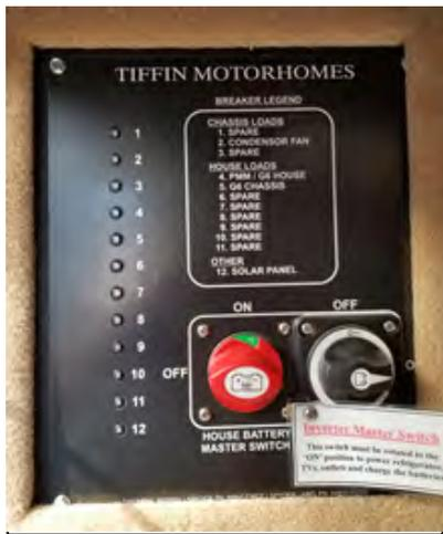
Figure 8-6: 12 VDC disconnect switch
