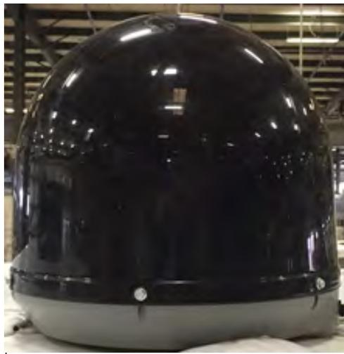
Figure 5-2: The dome satellite on top of the motorhome can be raised allowing easy access to change switches to a new satellite provider.
