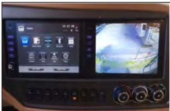
Figure 14-1: Xcite radio and camera monitor
