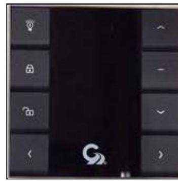
Figure 13-2: Awning control switch
