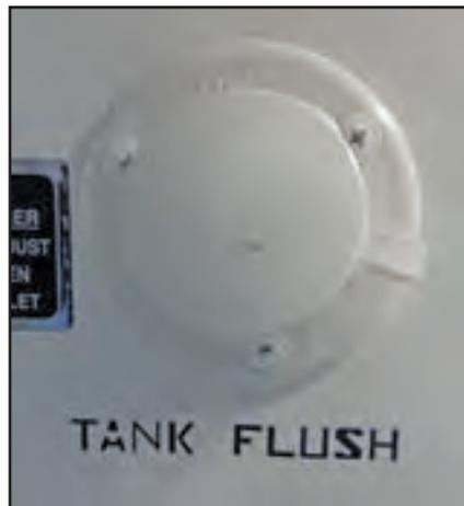
This vehicle may be equipped with a flushing system for the black-water holding tank. When draining your sewer tank, attach a water hose to the tank flush connection (Figure 12-12). After the tank is drained, leave the gate valve “open” and open the water valve to allow water to spray inside the black-water tank. This will clean the inside of the tank of any debris that may be left inside the tank. After this procedure is done, disconnect the freshwater hose and close the gate valve.
