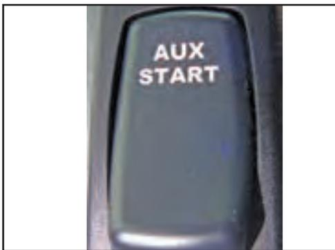
Figure 8-2: Auxiliary start switch
