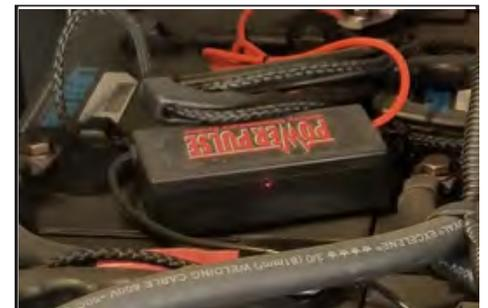
Figure 8-7: Battery maintainer
