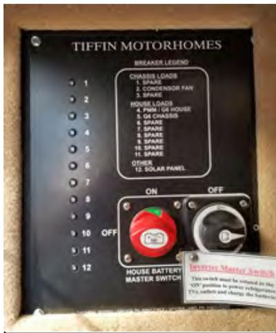
Figure 8-6: 12 VDC disconnect switch
