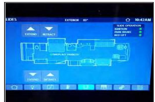
Figure 9-1: Slide-out screen on the Spyder control system
