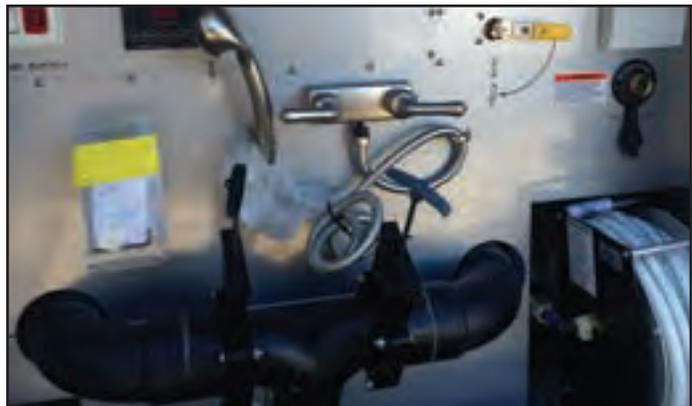
Figure 12-11: Sanitation coupling, valve, and hose
