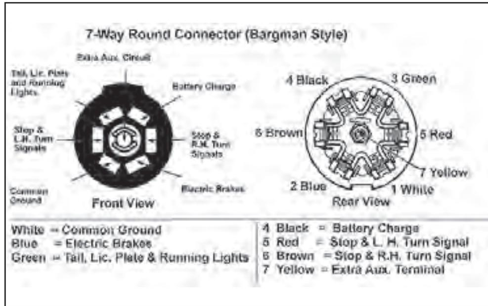
Figure 8-17: Seven-Pin towing connector
