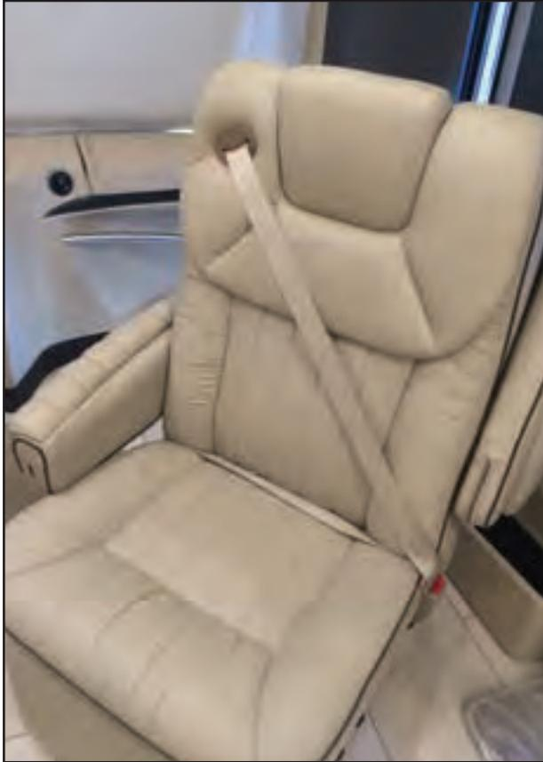
The driver's seat is manually operated and has swivel features. When the motorhome is parked, the driver's seat can be swiveled to face into the living room. To swivel this chair, first extend the slide-out room. Then move the chair backward as far as possible to gain clearance from the steering wheel. Now the chair can be swiveled without interference.
