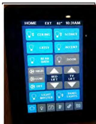
Figure 5-7: Rear TV lift on 5" touch screen
