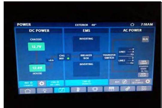
Figure 8-11: Converter/Inverter control screen
