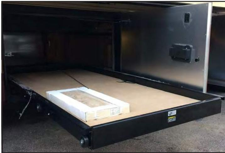
Figure 9-2: Extended Electric Cargo Tray
