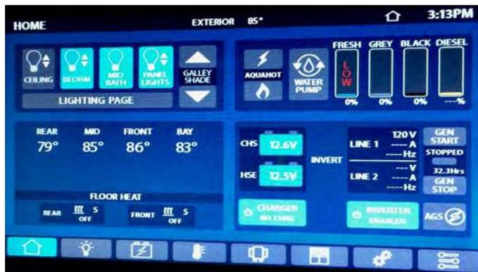
Figure 12-3: Tank level monitor on the 10" touch panel in hallway
