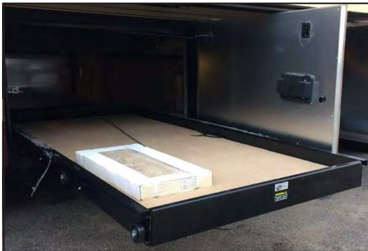
Figure 9-2: Extended Electric Cargo Tray
