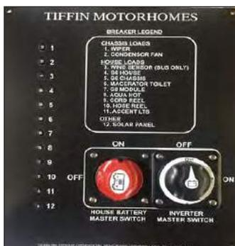
Figure 8-4: House battery disconnect panel switch
