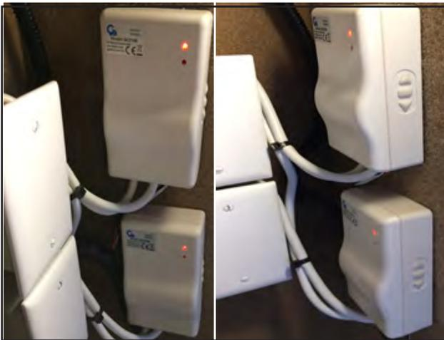
Figure 13-3: Awning modules located in the cargo bay
