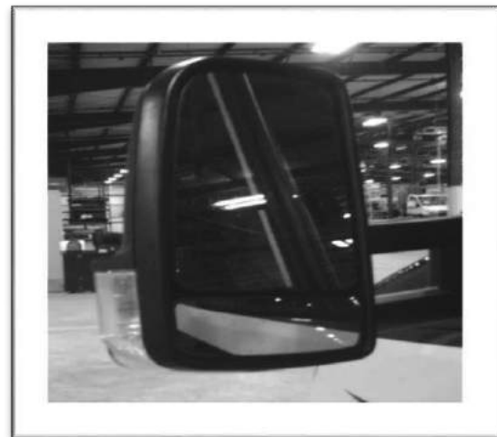
Figure 11-6: Mirror Move the control in the direction of movement desired to obtain the best view for that mirror. The adjustment control moves the top half of both
