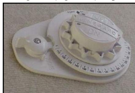
Figure 4-7. TV Satellite Dish Controller
