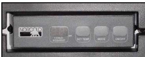
Figure 4-2. Norcold Refrigerator Control Panel
