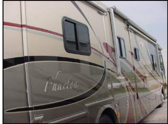
Figure 13-4. Awning (Fully Retracted)
