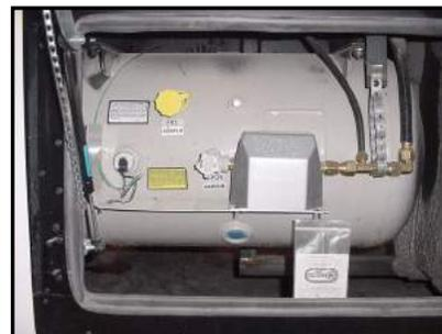
Figure 3-3. Liquid Propane Tank
