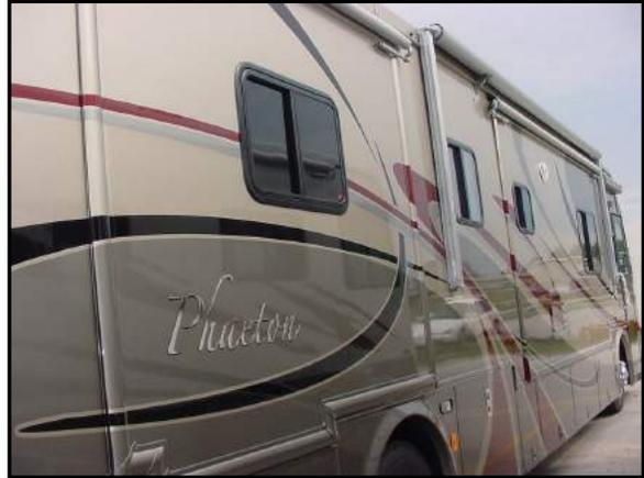
Figure 13-4. Awning (Fully Retracted)
