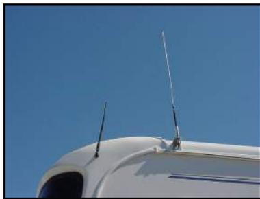
Figure 4-17. CB Radio Antenna
