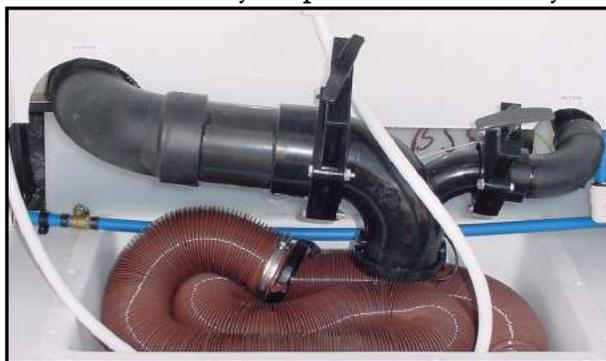
Figure 11-10. Sanitation Coupling, Valve, and Hose
