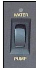
Figure 11-5. Water Pump Switch
