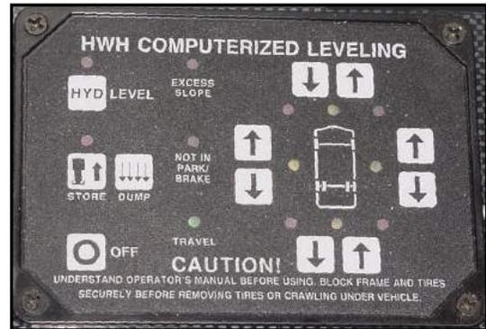
Figure 9-5. HWH Computerized Leveling System
