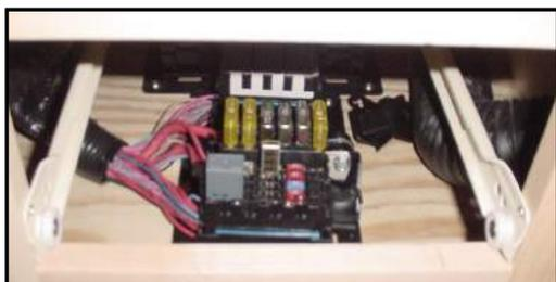
Figure 7-21. Fuse Blocks within Center Console
