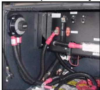
Figure 7-6. Engine Battery Disconnect Switch (left side)
