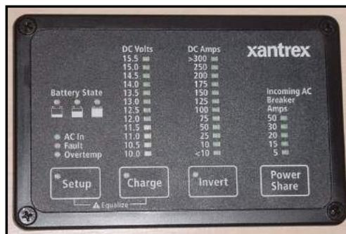
Figure 7-15. Inverter Control Panel
