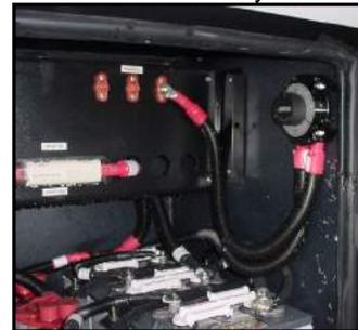
Figure 7-7. House Battery Disconnect Switch (right side)
