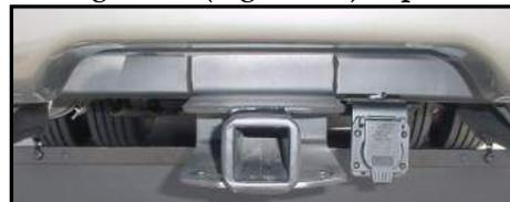
Figure 9-1. Towing Hitch
