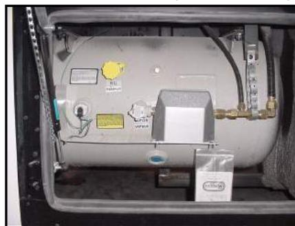
Figure 2-4. Liquid Propane Tank
