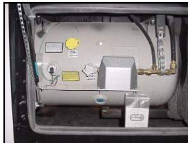
Figure 2-3. Liquid Propane Tank
