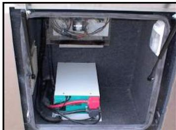
Figure 7-14. Inverter/Converter (Optional)
