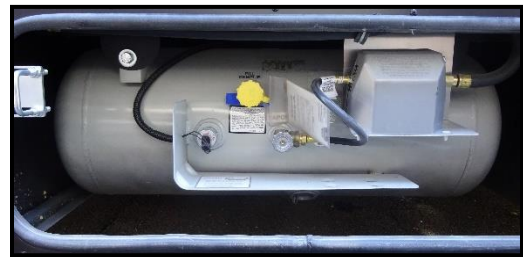
Figure 2-2: LP Tank and Regulator
