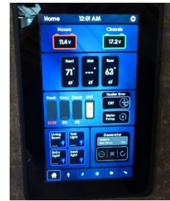
SPYDER Control showing approximate amount of LP Gas Remaining in Tank.
