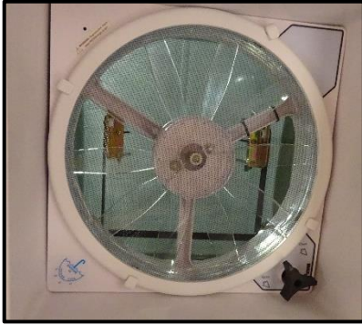
Figure 14-3: Overhead Vent Fan
