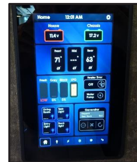
Figure 9-16: Multiplex System Switch Panel
