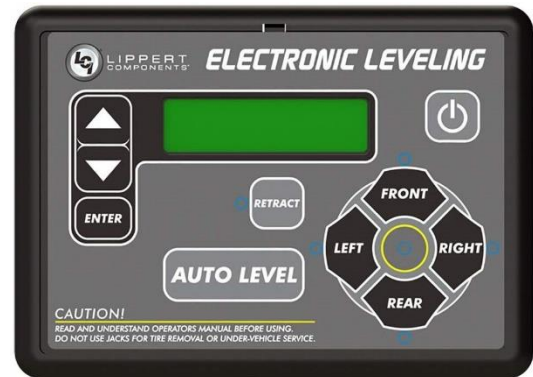
Figure 15-5a: Lippert Control Panel
