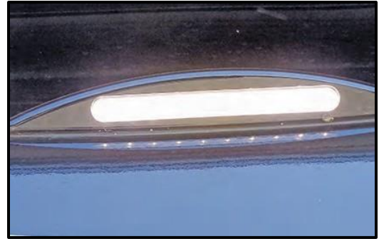
Figure 11-3: Exterior Security Light
