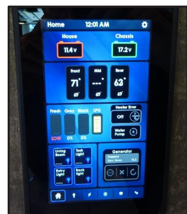
Figure 13-5: Spider Controls System Switch
