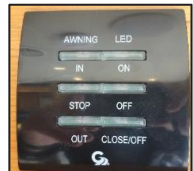
Figure 14-3: Patio Awning Control Switch
