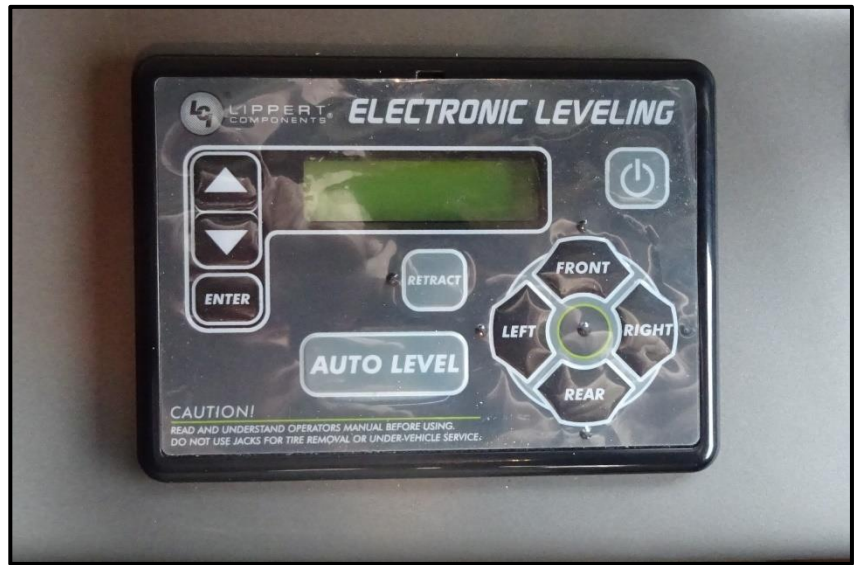
Figure 15-5: Leveling System Control Panel
