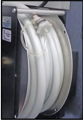
Figure 13-6: Motorhome Water Hose
