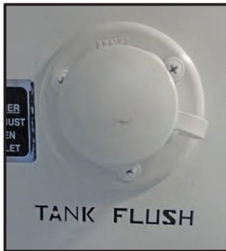
Figure 13-12: Tank Flush Connection
