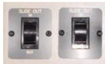
Figure 8-1. Slide-Out Switches
