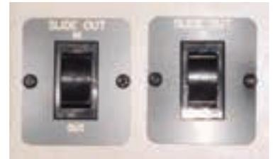
Figure 8-1. Slide-Out Switches
