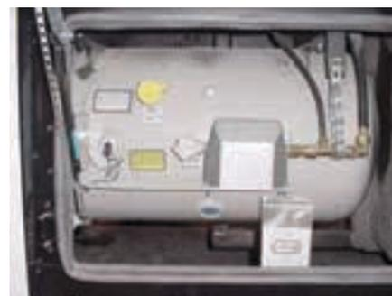
Figure 3-4. Liquid Propane Tank
