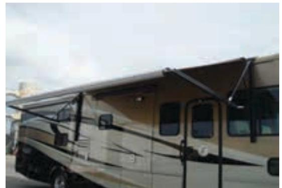
Figure 12-3. Power Patio Awning (Fully Extended)
