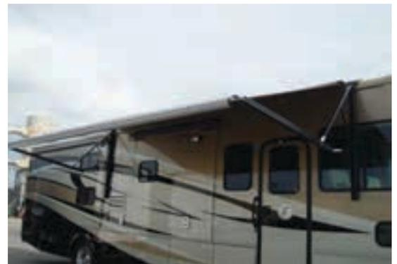
Figure 12-3. Power Patio Awning (Fully Extended)
