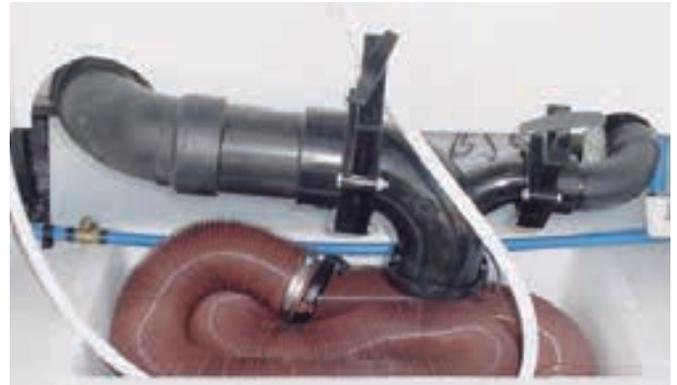
Figure 11-11. Sanitation Coupling, Valve and Hose
