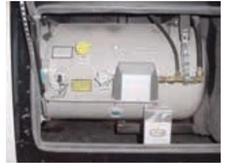
Figure 2-3. Liquid Propane Tank
