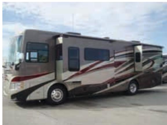
Figure 8-2. Typical Slide-Out Fully Extended
