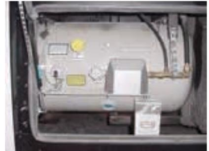
Figure 2-5. Liquid Propane Tank
