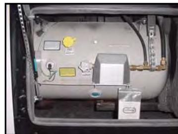
Figure 2-5. Liquid Propane Tank
