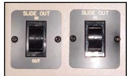
Figure 8-1. Slide-Out Switches
