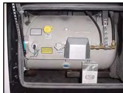
**Figure 3-4. Liquid Propane Tank**
