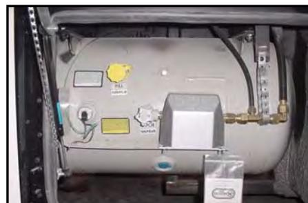
Figure 2-3. Liquid Propane Tank
