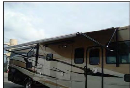
Figure 12-3. Power Patio Awning (Fully Extended)
