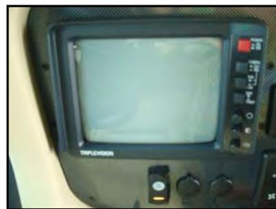
Figure 4-19. Rear-View Camera Monitor System
