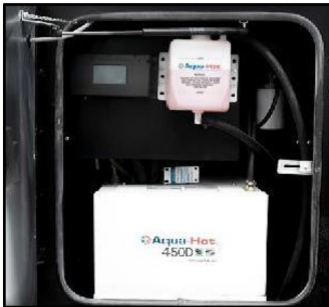
Figure 4-2: Aqua-Hot Surge Tank
