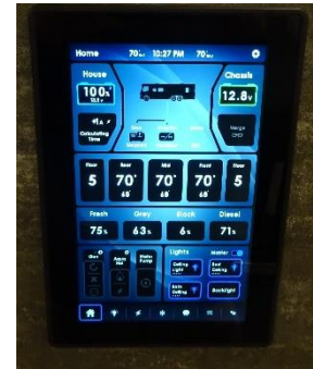
Figure 3-2: Home Screen for the Spyder Controls System
