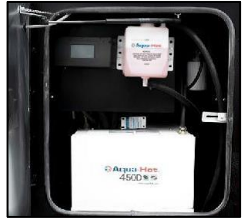
Figure 13-17: Aqua-Hot Surge Tank
