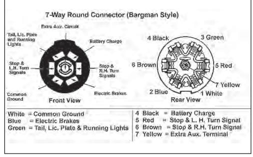
Figure 9-17: Seven-Pin towing connector
