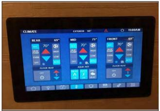
Figure 4-6: A/C Thermostat Control page on 5" panel
