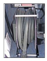
Figure 9-15: Electrical power cord reel
