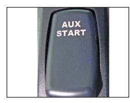
Figure 9-2: Auxiliary start switch
