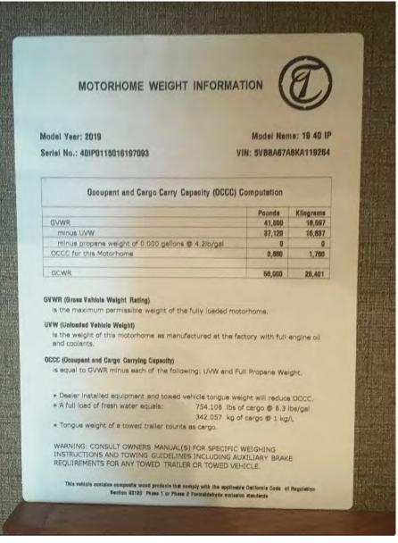
Figure 1-4: Sample Motorhome Weight Label located in the bedroom closet
