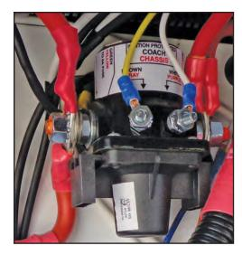
Figure 9-6: 12 VDC disconnect switch
