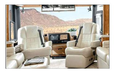
Figure 7-7: Both the driver's and passengers chairs swivel to face the living area of the coach.
