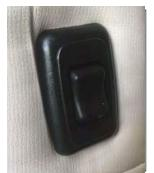
Figure 10-2: Slide-out switch on passenger and driver seat
