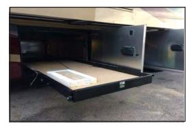
Figure 11-3: Extended Electric Cargo Tray
