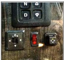
Figure 11-10: Mirror adjustment controls
