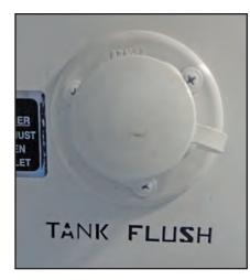
This vehicle may be equipped with a flushing system for the black-water holding tank (Figure 13-12). When draining your sewer tank, attach a water hose to the tank flush connection. After the tank is drained, leave the gate valve "open" and open the water valve to allow water to spray inside the black-water tank. This will clean the inside of the tank of any debris that may be left inside the tank. After this procedure is done, disconnect the freshwater hose and close the gate valve.
