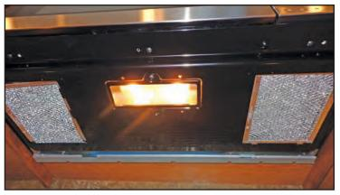
Figure 5-4: Air filtration fan In the Allegro Bus, the "exhaust" or airfiltration fan (Figure 5-4) is built into the microwave and its function is to filter the air and exhaust to the outside. The filtration fan should be used whenever any cooking is performed to filter any airborne cooking residues and heated air.
