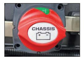
Figure 9-5: Engine battery disconnect panel switch
