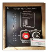
Figure 9-4: House battery disconnect panel switch
