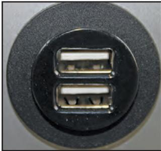
The Allegro Bus is equipped with USB ports conveniently located on the front dashboard and in the bedroom area as well as on the passenger console. These ports allow for easy access when charging cell phones, laptop computers, iPods, iPads or other tablets.
