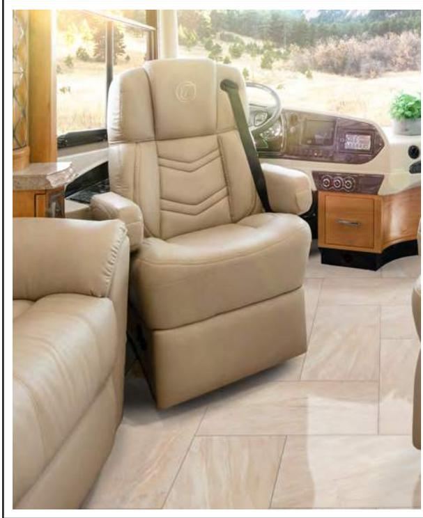
Figure 7-7: Both the driver's and passengers chairs swivel to face the living area of the coach.
