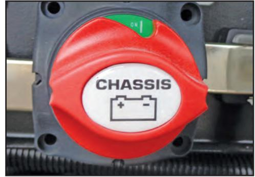
Figure 9-5: Engine battery disconnect panel switch
