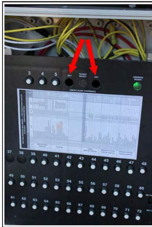
Figure 10-4 : Location of Slide-out room control override
