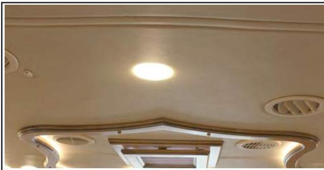
The ceiling (Figure 12-4) in the Allegro Bus motorhome is covered with a padded vinyl headliner which can be easily cleaned with a damp, soft cloth and a mild detergent.
