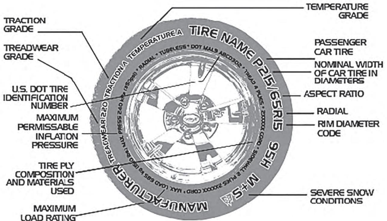
**P**—The “P” indicates the tire is for passenger vehicles. **NOTE:** Passenger car tires are not recommended for use on trailers, because the capacity ratings are not marked on the side walls of these tires. In the event a passenger car tire is used, the capacity must be de-rated by 10%.
