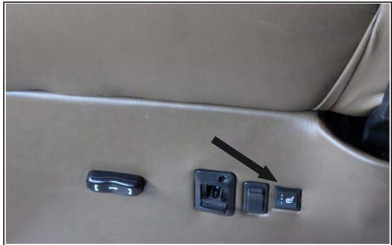
Figure 7-8: Heated Seat Switch
