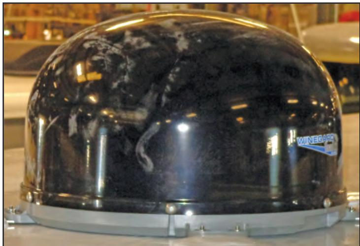
Figure 6-2: The dome satellite on top of the motorhome can be raised allowing easy access to change switches to a new satellite provider.
