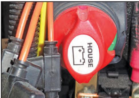
Figure 9-4: House battery disconnect panel switch
