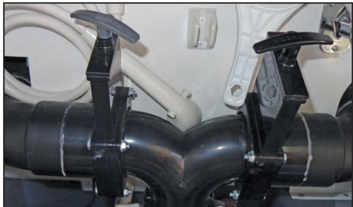
Figure 13-10 :: Sanitation Coupling
