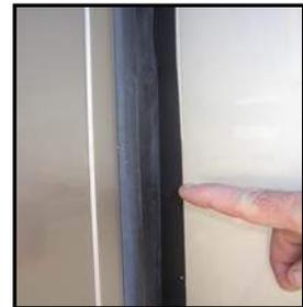
**Figure 14-6. Inspecting Slide Out Gasket**
