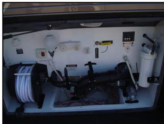
Figure 11-13. Sanitation Compartment Containing Holding Tank Drains and Flexible Drain Hose
