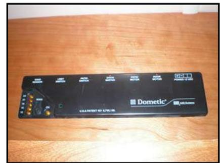
Figure 13-2. Dometic Awning Control Box
