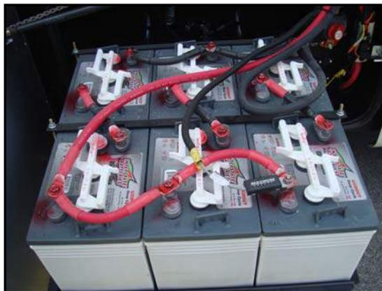
Figure 7-6. Battery Slide Tray
