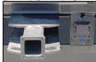
Figure 9-1. Towing Hitch
