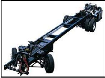
Figure 12-1. Freightliner Chassis
