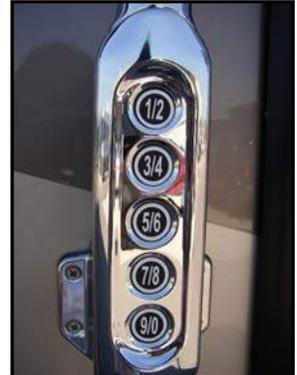
**Figure 13-8. Detail of Keyless Lock**
