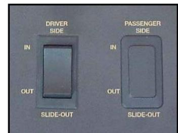
Figure 8-1. Slide-Out Switches
