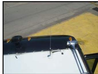
Figure 4-21. CB Antenna Installation
