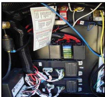
Figure 7-2. 12 VDC Fuse Panels
