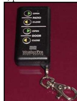
**Figure 13-3. Dometic Awning Key Fob Controller**
