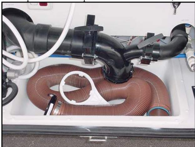
Figure 11-14. Sewer Hose and Drain Connections
