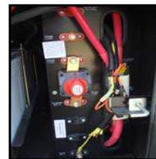
Figure 7-9. Rotary Switch to Disconnect “House” Batteries
