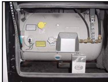
Figure 2-3. Liquid Propane Tank
