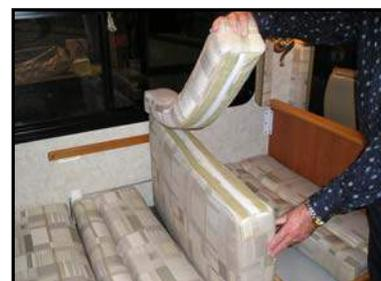
Figure 5-5. Filler Strip Attached to the Seat Portion
