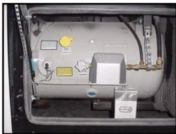
**Figure 3-7 Liquid Propane Tank**
