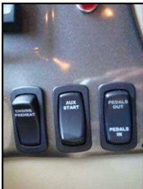
**Figure 7-3. Auxiliary Start Switch (Center)**
