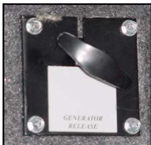
Figure 7-18. “Pull” Cable for Generator Release
