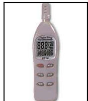
**Figure 14-5. Portable Hygrometer**
