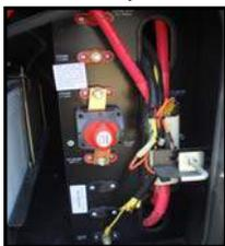
Figure 7-8. Rotary Switch to Disconnect Engine Battery
