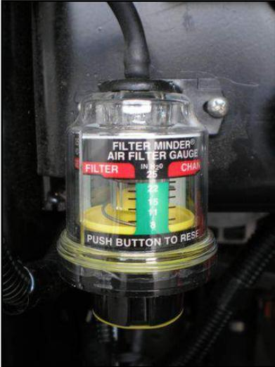
Figure 6-1: Filter Restriction Indicator
