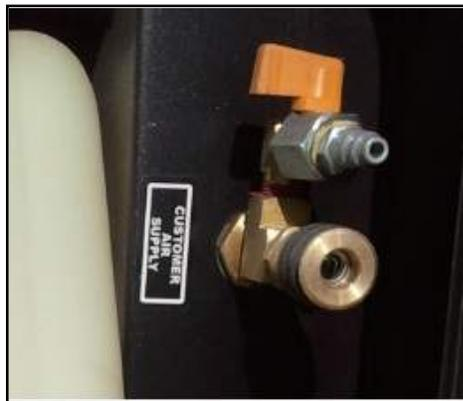
Figure 8-2: Rear Customer Air Supply
