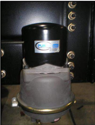
Figure 3-3: Haldex Purest Air Dryer
