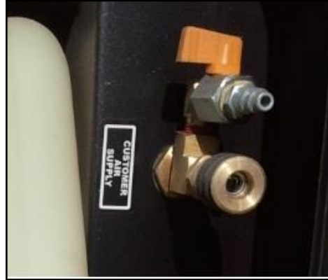
Figure 8-2: Rear Customer Air Supply
