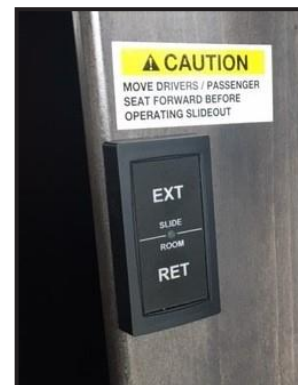
Figure 10-2: Front Slide-Out Switch
