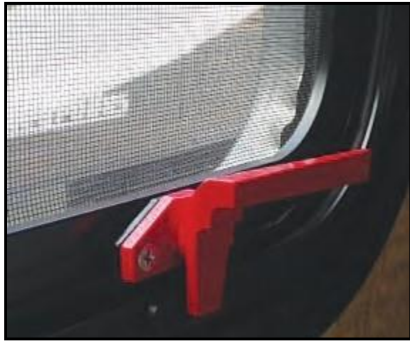
Figure 2-9: Emergency Exit Latch
