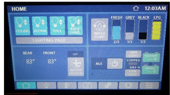
Figure 3-1: Spyder Controls System
