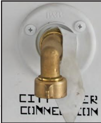
Figure 13-7: City Water Supply Connection
