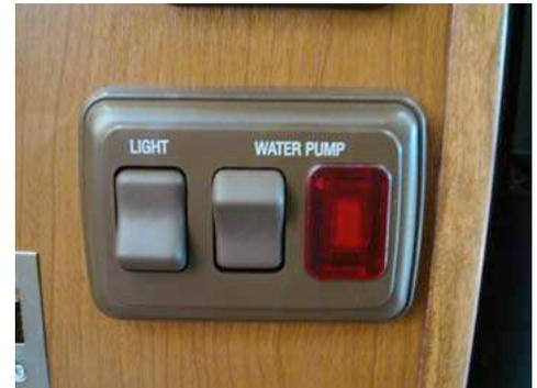
Figure 11-5. Water Pump Switch
