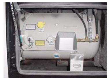
Figure 3-4. Liquid Propane Tank
