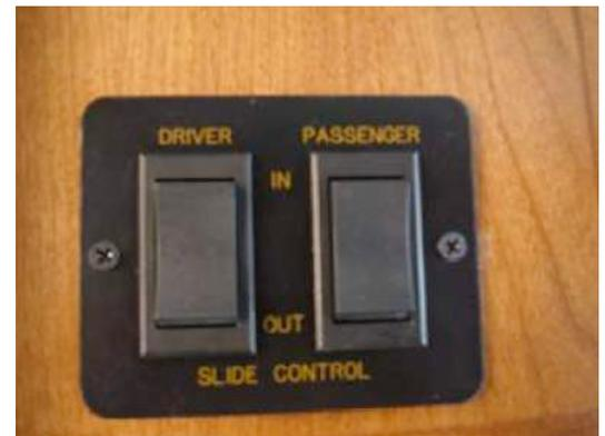
Figure 8-1. Slide-Out Switches
