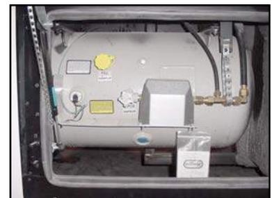
Figure 2-3. Liquid Propane Tank
