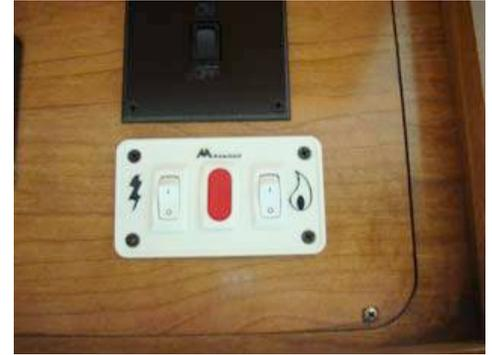
Figure 4-12. Water Heater Switches
