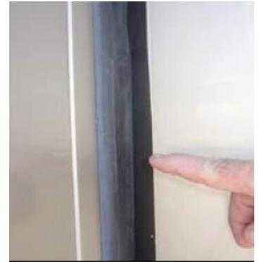
Figure 13-6. Inspecting Slide Out Gasket
