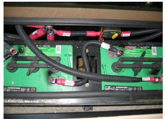
Figure 7-4. House Batteries (Underneath Entrance Door Step Well)
