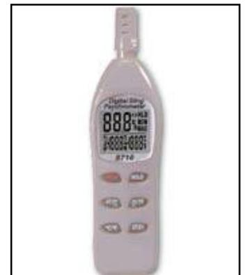
Figure 13-4. Portable Hygrometer
