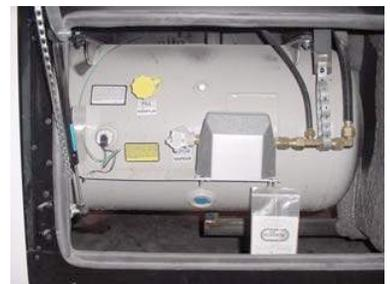
Figure 2-4. Liquid Propane Tank
