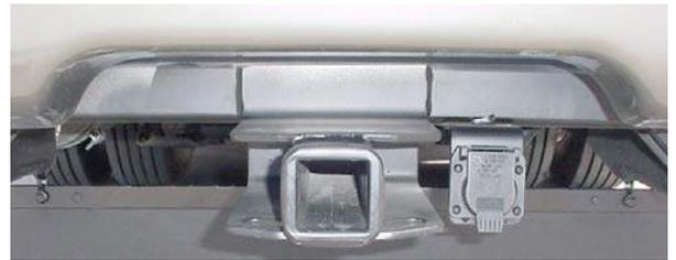
Figure 2-9. Towing Hitch
