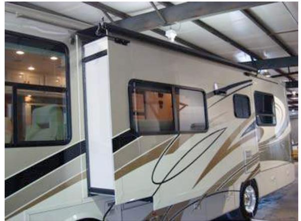
Figure 8-2. Typical Allegro Bus Slide-Out
