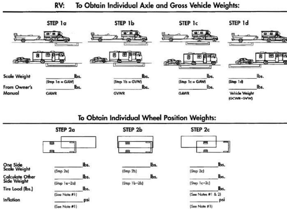
Figure 13-7. Procedure for Weighing the Motor Home (Each Tire Position Individually)
