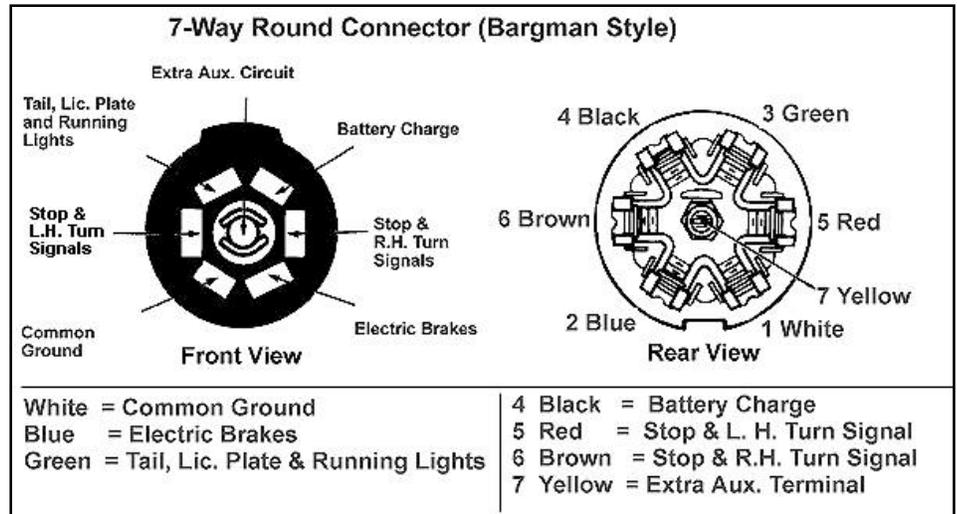
Figure 7-11. Seven-Pin Towing Connector
