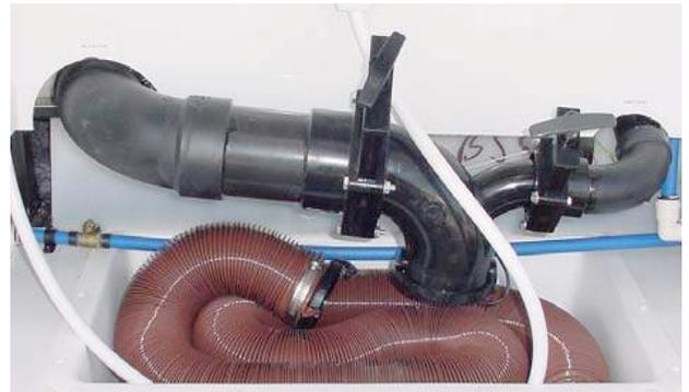
Figure 11-11. Sanitation Coupling, Valve and Hose
