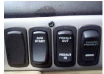
Figure 7-2. Auxiliary Start Switch
