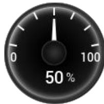
**DEF Temperature** - This gauge displays the temperature of the fluid in the Diesel Exhaust Fluid (DEF) tank.
