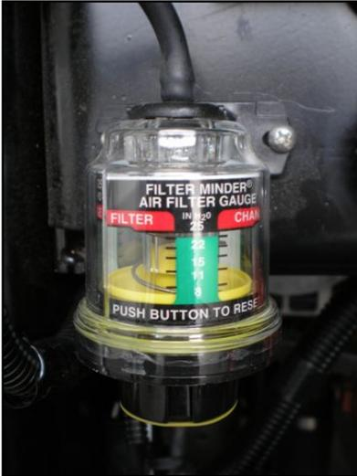
Figure 4-1: Filter Restriction Indicator
