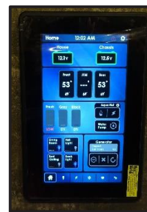
Figure 13-5: Spider Controls System Switch
