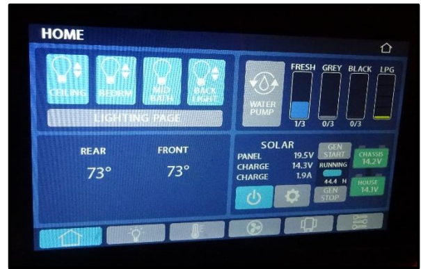
Figure 9-1: Spyder Controls System
