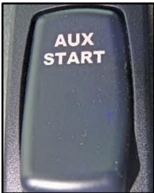
Figure 9-16: Auxiliary Start Switch
